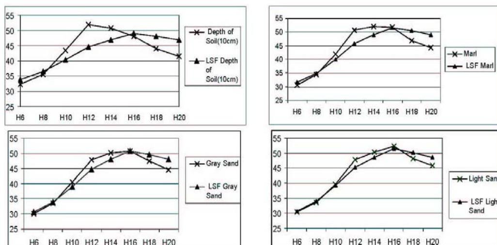
**Figure 4.** The comparison of real temperature and estimated temperature according to Least Square Fitting (LSF), Y-axis presents temperature in Celsius ( $^{\circ}$  C) and X-axis also presents times in every two hours during a day between 6 a.m. until 8 p.m..
